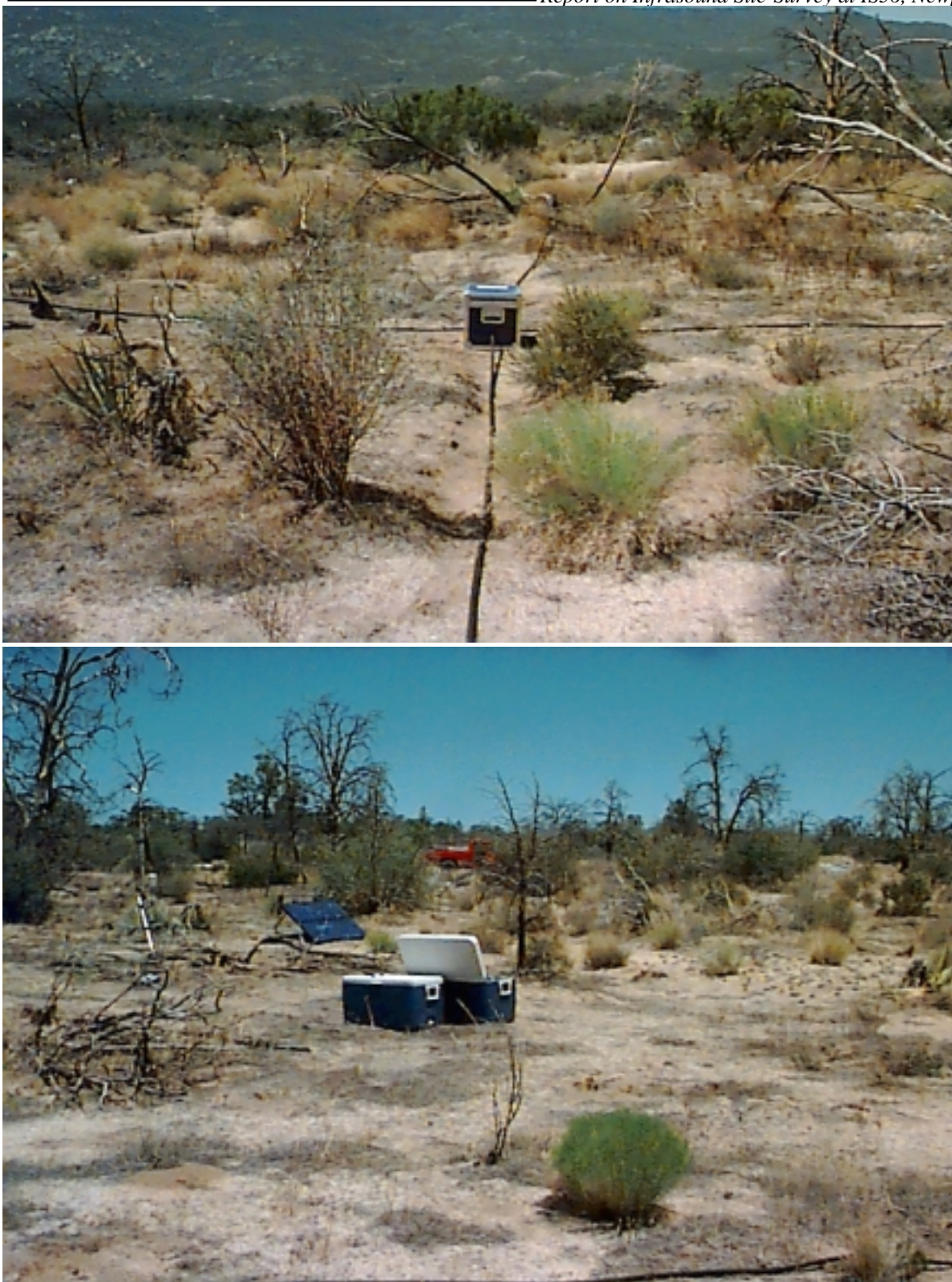
Figure C.1. The microbarometer and space filter deployed at site 4 in the Pinon Flat survey is shown in the photo at the top. The recording system enclosures are shown in the lower photo. To the left is the mast with the met sensors and the solar panel.
