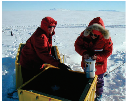
The Model 5.1 is installed inside a plastic vault at IS55, Antarctica.
